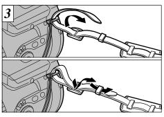
Attach the shoulder strap to the strap mounts. After attaching the shoulder strap, check carefully that the strap is firmly secured.
